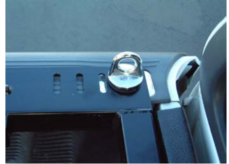
Fig 7. Shield inserted in tie-down Fig 8. Stake pocket assembly and islet Fig 9. Islet screwed into stake pocket
