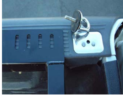
Fig 7. Shield inserted in tie-down Fig 8. Stake pocket assembly and islet Fig 9. Islet screwed into stake pocket
