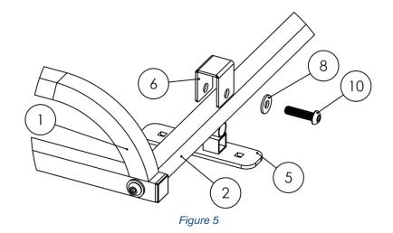
6. Install the rear Feet. Repeat Step 5 by attaching the U-Shaped Clamp (Item No. 6) and the Feet (Item No. 5) onto the rear Crossbar B (Item No. 3). Again, make sure that the thread found on the Clamp is on the opposite side of the Screw insertion and that the long end of the Feet point toward the front Feet. Tighten both rear Clamps once you have marked the top of your canopy through the holes in each Foot.
