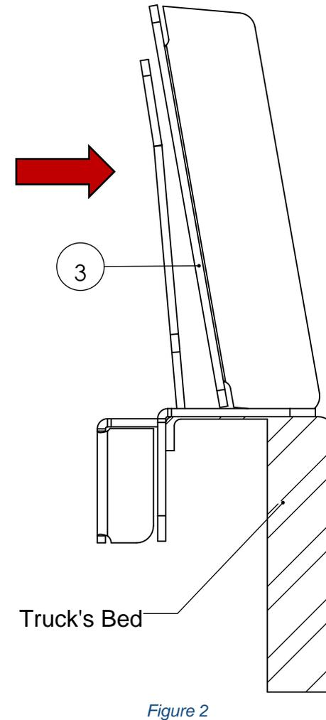
1. **Position the base of the rack.** To install the rack's base, you must first place each Base Rail Assembly (**Item No. 3**) correctly on the bed rail. Examine each one and locate an oval shaped eyelet on the gusset. These eyelets should be positioned so that they face each other as shown in **Figure 1**. Complete the positioning by sliding the Base Rail Assembly onto your truck's bed as shown in **Figure 2**. Keep in mind that the distance between the Base Rails is at your discretion.
