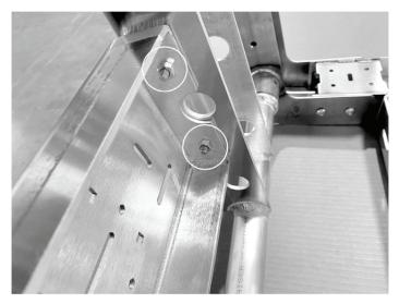
8. Close the gate door and lock into legs using (4) supplied pins. Install the accessory mount panel as shown using (4) 1/4" x 3/4" hex bolts, washer and nuts.
