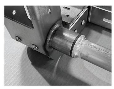
5. Install the gate shaft bushing into the leg housing as shown for both sides of the rack. Confirm gate shaft and leg numbers match.
