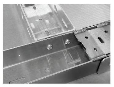
6. Connect second side of both of the lateral cross bars to the transverse cross bar as shown. Torque to 30 ft/lb.
