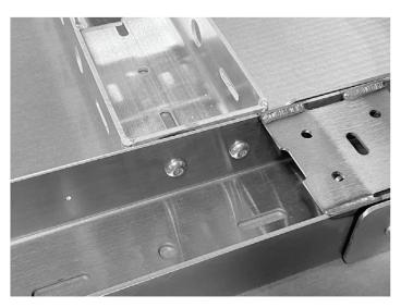
3. Connect one side of both of the lateral cross bar as shown. Torque to 30 ft/lb.
