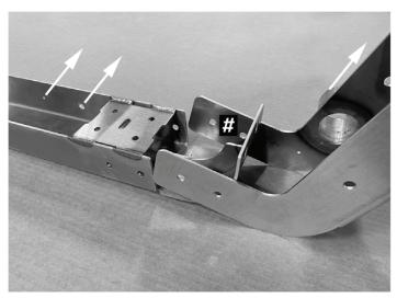
1. Install each leg to the transverse cross member. Use (8) 3/8"x1" button head bolts and flange nuts for each corner. Do not tighten securely. Make sure holes on cross member and gate pivot tube are facing the lateral cross member in the next step. Take note of the number mark on the leg flange.
