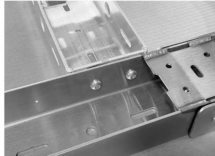
3. Connect one side of both of the longitudinal cross bar as shown. Use (2) 3/8"x1.25" button head bolts and flange lock nuts. Torque to 30 ft/lb.
