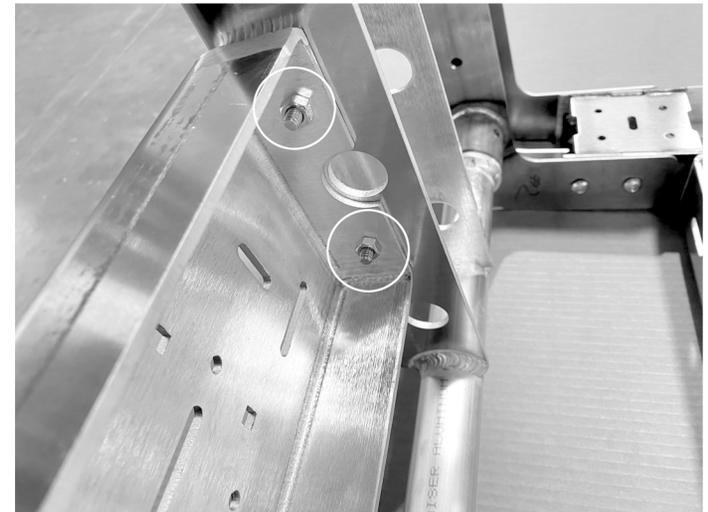
7. Close the gate door and lock into legs using (4) supplied pins. Install the accessory mount panel as shown using (4) 1/4" x 3/4" hex bolts, washer and nuts.
