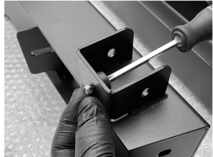
6. Install the rubber stop to each of the (4) legs. Use (1) 6-32 x 3/4" machine screw and (1) 6-32 nylon lock nut for each stop.
