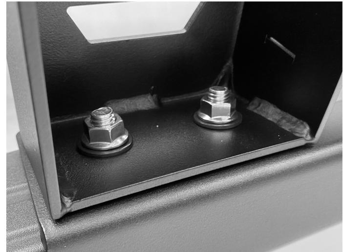
15. Use (2) 3/8" hex lock nuts and (2) flat washers to secure the legs of the rack to the base rails. Secure the clamp bolts under the rail to the bed (From step 11.) to secure the rail to the vehicle.
