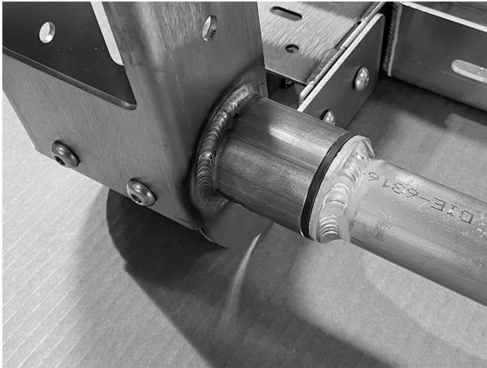
4. Install the gate shaft bushing into the leg housing as shown for both sides of the rack. Install the gate shaft into the bushing. Repeat for opposite side.
