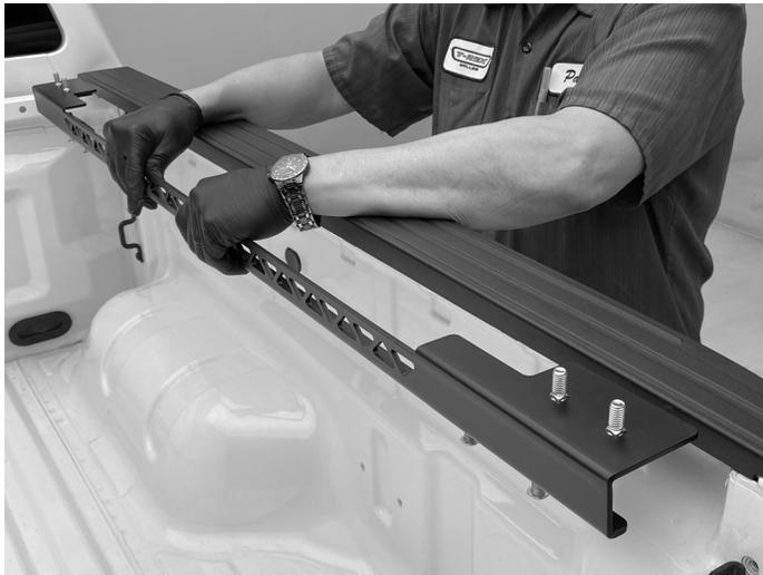
13. Install the passenger side base rail as shown. Do not tighten the clamp bolts under the rail at this time.
