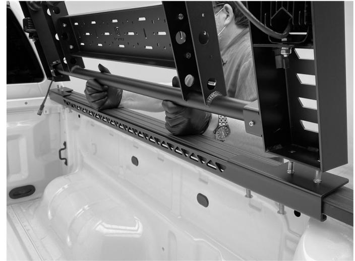
14. Install the rack to the base rails as shown. Center the rack in the bed.
