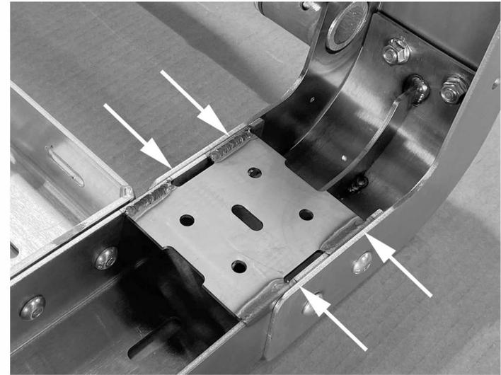
2. Align the leg with the transverse cross bar and tighten all fasteners. Torque to 30 ft/lb. Confirm leg flanges are parallel with cross bar as shown.
