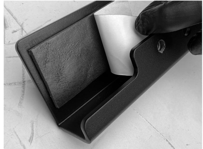
10. Cut (4) pieces of foam and attach adhesive side towards the rail to retain the bolts.
