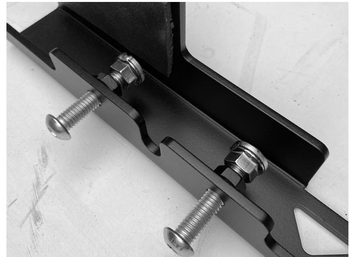
11. Install (8) 2" button cap bolts into each of the (2) rails as shown. Once the thread passes through, install the welded nut with the cap on each bolt. Make sure the bolt is only far enough through to install the nut in order to clear the bed rail of the truck during installation.
