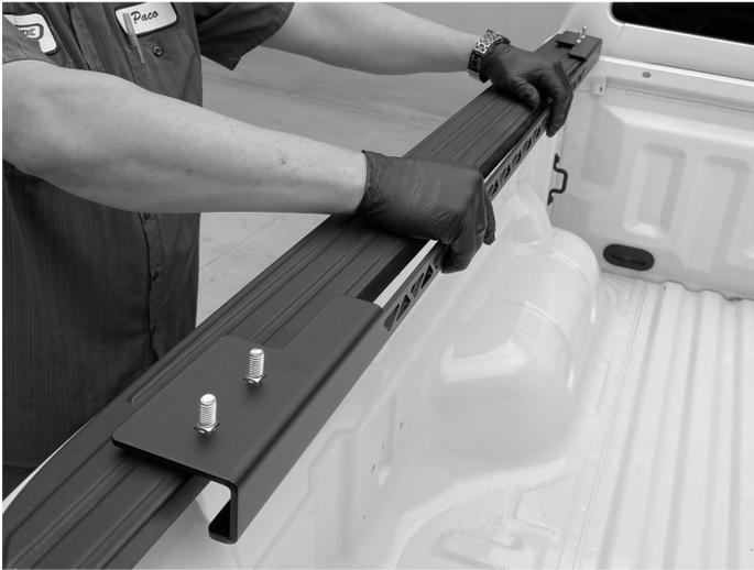
12. Install the driver side base rail as shown. Do not tighten the clamp bolts under the rail at this time.
