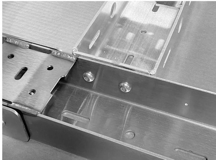
5. Connect the opposite side longitudinal cross bar as shown. Use (2) 3/8"x1.25" button head bolts and flange lock nuts. Torque to 30 ft/lb. Install the harness bracket as shown, use (2) 3/8" flange lock nuts, Torque to 30 ft/lb.
